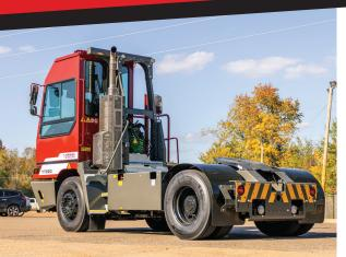
The YT220 Yard Tractor can, on average, move three trailers in the time it would take to move one with a conventional Class 8 trucks.
